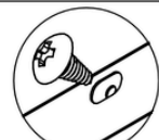
Bolt the left side and back plate with self-tapping screws(S5x10)
