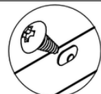
Attach the left side to the back panel using self-tapping screws (5×10).
