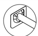
Install the bottom panel, then fix the divider panel as indicated.
